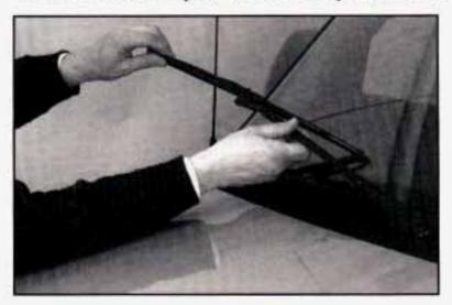
To replace your windshield wiper blade inserts, lift the wiper arm away from the windshield. Pinch the two tabs on the wiper arm and slide the insert out of the blade. Slide the new one in place. Make sure the tabs are locked into position.
